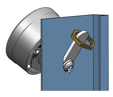
2. Assembly sequence for cams to be retrofitted
