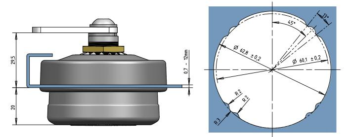
2. Recessed installation in wooden doors using special milling and optional installation shell (Specify when ordering)
